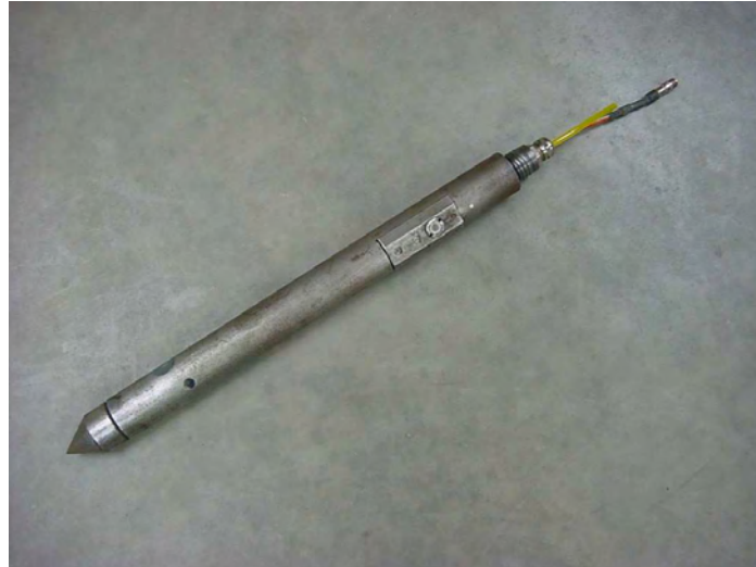
Figure 2. HPT Probe. A small injection screen is located near the top of the probe, and an electrical conductivity dipole is located near the tip.
