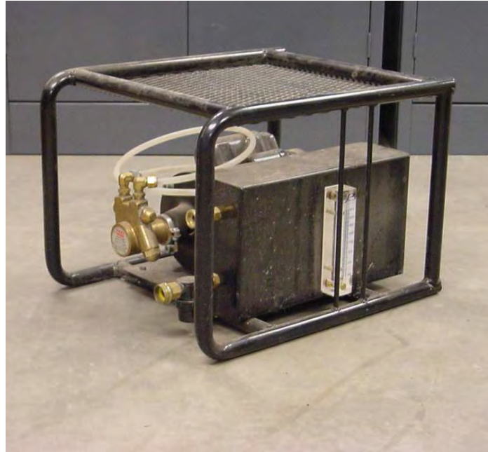
Figure 4. HPT Pump. System pressure is increased to maintain flow to the probe.
