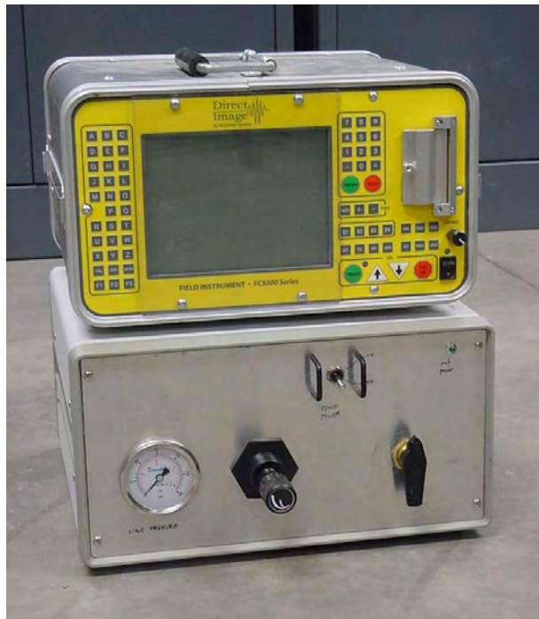
Figure 3. HPT Controller and Field Computer. The controller regulates and monitors water injection, while the required parameters are displayed and saved on the field computer.
